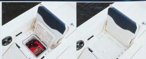
Two comfortable jump seats open for rear storage and fold flat for a larger stern casting area.
