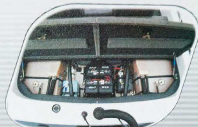
Easy Access Rigging Compartment with ZX Tandem Fuel Tanks
