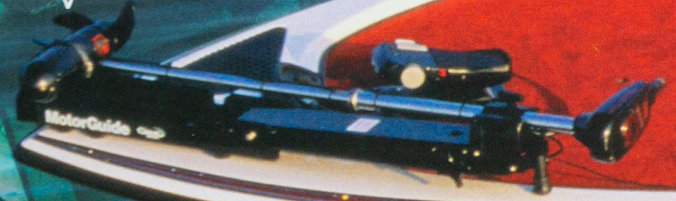
MotorGuide® 24v trolling motors with Gator mounts
