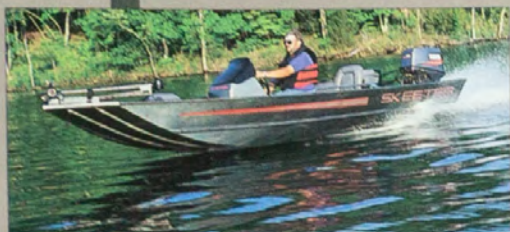
Centerline - 17'0" Beam - 69" Fuel Capacity - 16 gals. Max. Hp - 75
