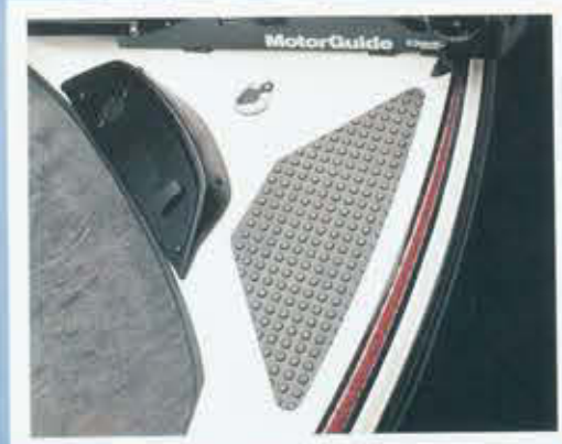
The new bow traction mat design with Anti-Skid Grippers provides stability underfoot while boarding and launching.
