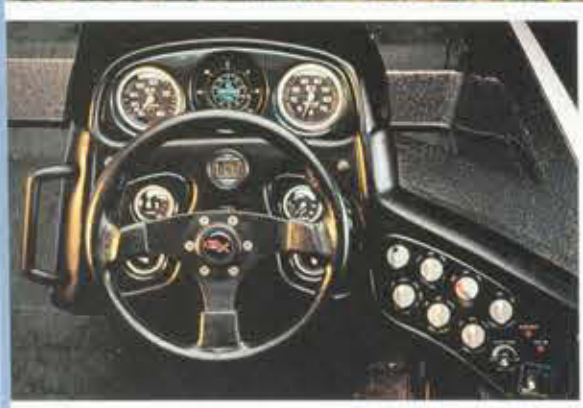
The new Techno Dash Cockpit Command Center features new Faria ZX Series screened gauges and lit rotary switches.
