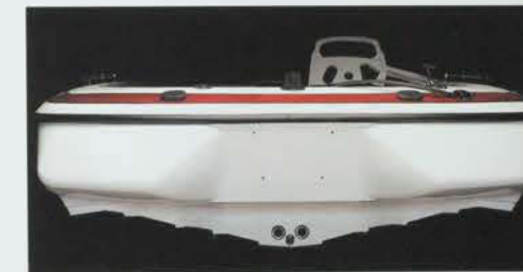
New Stretched Sponsons with a No-Splashwell Design Stern provide added lift and buoyancy and reduces backwash.
