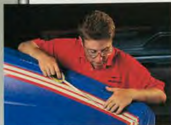
Precision hand-crafted hulls receive a S-stripe mask over primary gelcoat layers before a deep layer of poliflake and gelcoat are sprayed into the mold.
