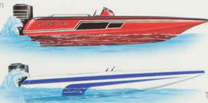
Our patented reverse draft transom adds buoyancy to ensure no back splash and a balanced boat from stern to bow.
