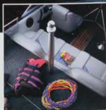
The easily removable, tournament-style ski tow pylon does not require supporting struts, leaving the rear deck unobstructed for sunbathing. (Sun pad optional.)
