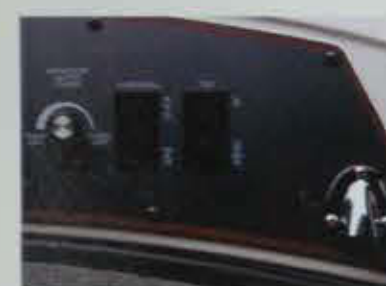
Engine tilt-trim switch and livewell timer on the bow panel are standard on the SS140.
