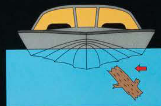
The hull design on all Skeeter models allows easy slip-off of underwater stumps and logs.
